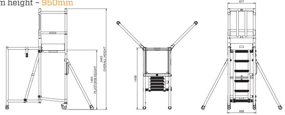
Maximum Safe Working Height\*: **3.45m**Maximum Safe Working Load: **150kg**Weight: **38kg** (excluding toe board kit)
